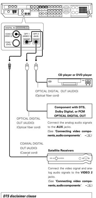
When playing DTS-encoded discs, excessive noise will be exhibited from the analog stereo outputs of the CD or DVD player. To enjoy DTS Digital Surround<sup>™</sup> playback, this unit must be connected to the digital output of the CD or DVD player.
