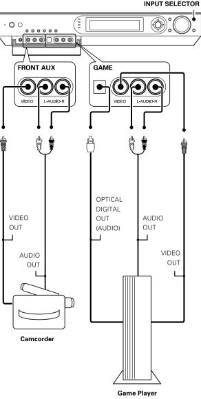
• The DIGITAL IN (OPTICAL) jack in the GAME jack section can be used for connection of digital audio input. This is convenient for playing a video game through the receiver.  $\rightarrow 21$
