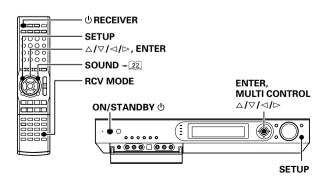
2 Turn on the power to this receiver by pressing the ON/ STANDBY ⊕ key (or the ⊕ RECEIVER ).
