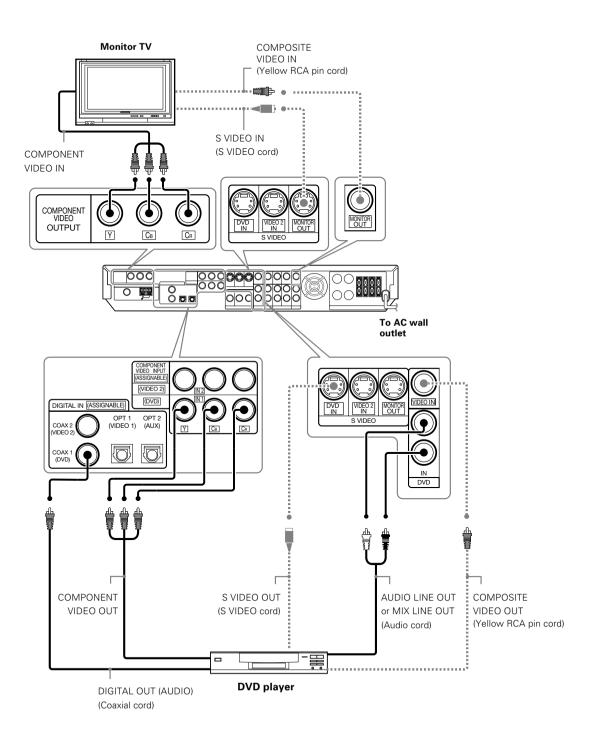
• Digital audio connections are required when playing multi-channel signals such as the Dolby Digital and DTS signals.
