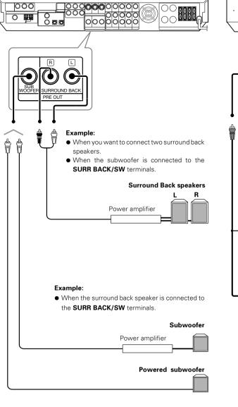
• Connecting a speaker cord directly to a PRE OUT jack will not produce any sound from the speaker.
